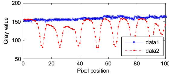
Fig. 2. Gray value distribution of pixels of portions of horizontal scan lines (data1 refers to the scan line across the background pixels, and data2 refers to the scan line across the stroke pixels).
