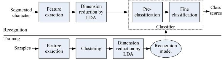
Fig. 4. Block diagram of the training and recognition process used in our system.
