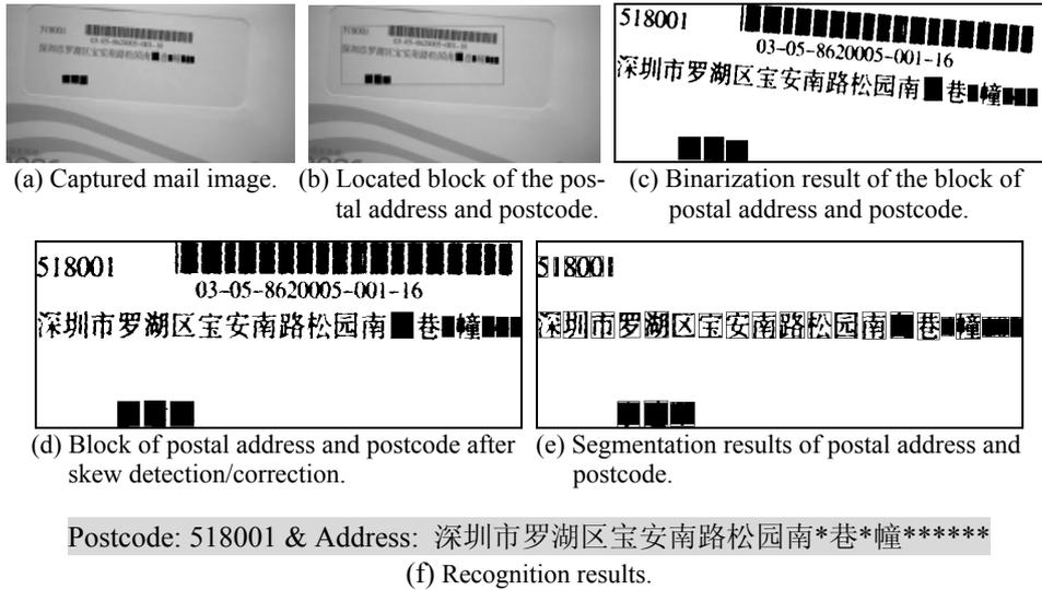
Fig. 6. Example of the mail image processing and recognition procedure used in our system. (From the image, the name of recipient and some detail address have been hidden to maintain privacy. The barcode on the top of image has been omitted in the processing of segmentation and recognition.)
