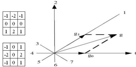
Fig. 3. Sobel operators and decomposing of the gradient vector.
