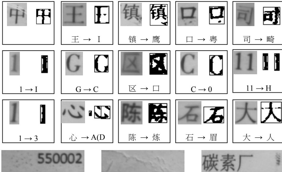
Fig. 7. Some typical examples of mis-segmentation and mis-recognition by our system. In each box, the top left shows the input character image (cropped from the envelope image for display), the top right is the segmented character produced by our system, and below are the ground truth and recognition results, respectively. The last row shows some examples of envelope images with dirty backgrounds.
